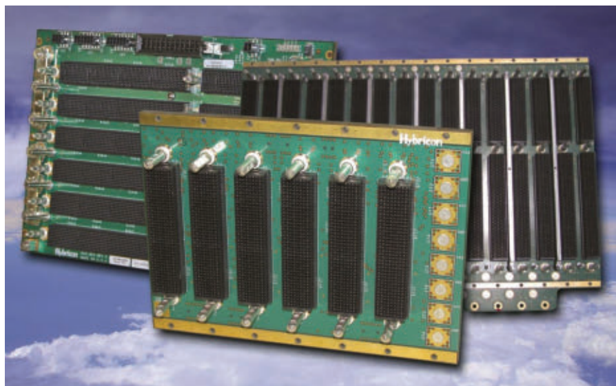
The Hybricon Fabric40 Backplane from Curtiss-Wright Defense Solutions offers 40-gigabit-per-second Gen3 OpenVPX 6U 6-slot embedded computing performance for the end-to-end transmission of high-speed data.
