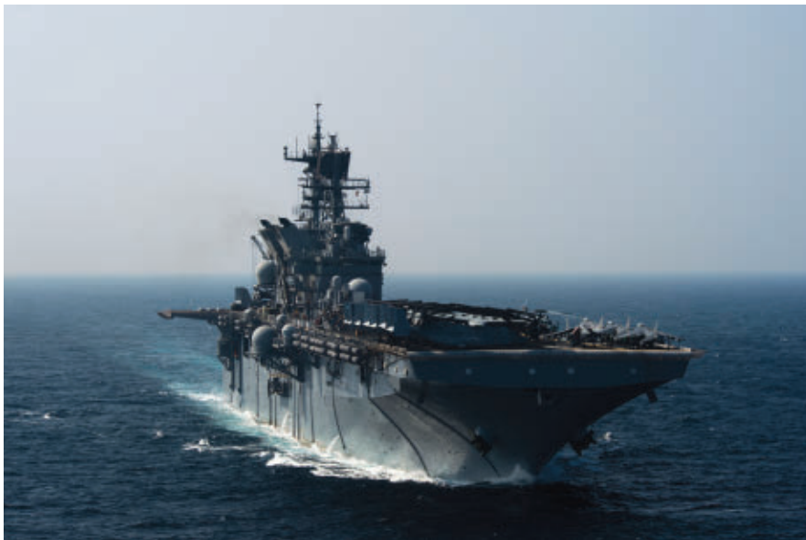
The amphibious assault ship USS Makin Island, shown above, introduced a hybrid conventional-electric drive propulsion system replicated aboard two subsequent amphibs serving as early steps towards full-up integrated electric drive for propulsion and ship power.
